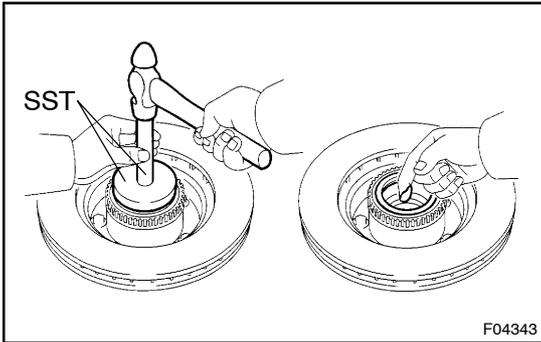
(b) Using SST and a hammer, install a new oil seal into the axle hub.
