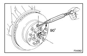
Using a spring tension gauge, measure the preload. (e)
