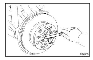
(d) Pull out the drive shaft outside the vehicle and select the snap ring which ensures the clearance between the tip of the flange and the snap ring is less than 0.2 mm (0.008 in.).
