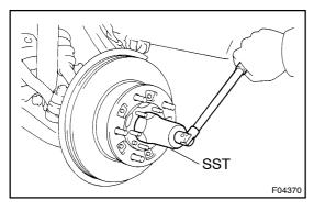
Using SST, torque the lock nut. (b)
