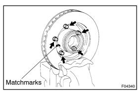
(b) Align the matchmarks and install the axle hub to the disc, and install the 5 bolts.
