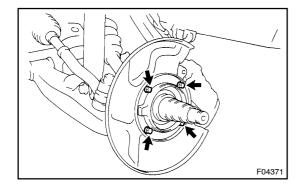
2. REMOVE OIL SEAL, GASKET AND DUST COVER
