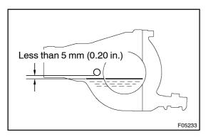
4. FILL DIFFERENTIAL WITH HYPOID GEAR OIL
