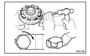
(g) Using a drift punch hammer, stake the 5 lock plates. HINT:
