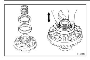
(c) Install outer races, adjusting nuts and sleeve to left side. HINT:
