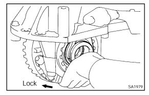
(i) Shift the fork deeply and keep the differential lock condition.
