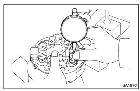
(e) Using a dial indicator, holding the side gear and spider, measure the side gear backlash,
