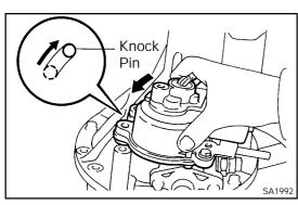
(f) Insert the actuator so that the long hole on the actuator side fits with the knock pin on the carrier side.
