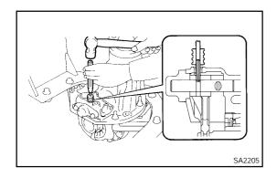
(h) Using a pin punch and hummer, install the slotted spring pin to the shift fork.
