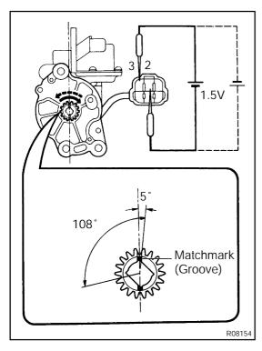
(b) Ensure that the matchmarks of the pinion of the actuator is between 0 and 5 degrees clockwise above the center line of the actuator.
