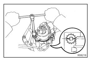
(h) Install the actuator to the differential carrier with the bolt so that the outermost positioned rack tooth of the shift fork will fit the matchmarks of the pinion of the actuator.
