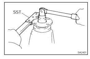
(c) Using SST to hold the flange, adjust the drive pinion preload by tightening the nut.
