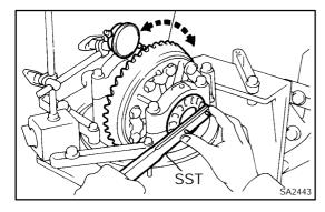
(h) Using a dial indicator, adjust the ring gear backlash until it is within the specification.
