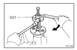
(b) Using SST, install the companion flange. SST 09950-30010 (09951-03010, 09953-03010, 09954-03010, 09955-03030, 09956-03020)
