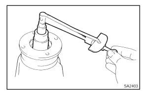
(k) Using a torque wrench, measure the preload.
