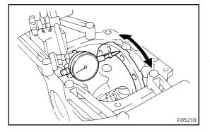
(f) Using a dial indicator, measure the differential case runout.
