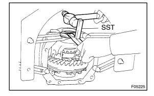
(c) Using SST and a hammer, remove the 2 side bearing plate washers.
