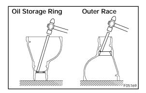
(b) Using a brass bar and hammer, remove the oil storage ring and front bearing outer race.
