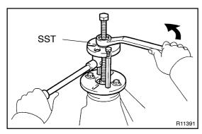
(c) Using SST, remove the companion flange. SST 09950 -30010 (09951 -03010, 09953 -03010, 09954-03010, 09955 -03030, 09956 -03020)
