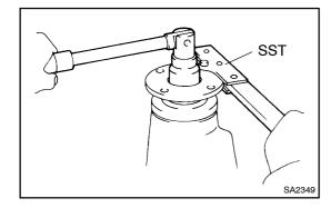
(b) Using SST to hold the flange, remove the nut. SST 09330 -00021
