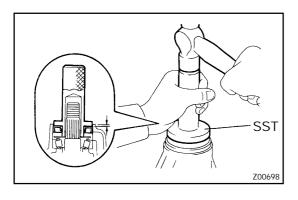
(b) Using SST and a hammer, install a new oil seal. SST 09554–30011
