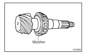
If the teeth are not contacting properly, use the following table to select a proper washer for correction.
