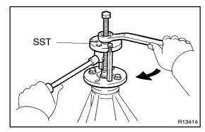
(c) Using SST, install the companion flange. SST 09950 -30010, (09951 -03010, 09953 -03010, 09954-03010, 09955 -03030, 09956 -03020)
