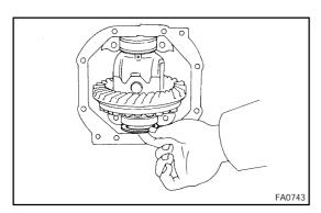
(d) Select a plate washer for back side ring gear, using the backlash as reference.
