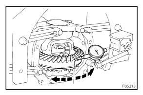
(f) Using a dial indicator, adjust the ring gear backlash until it is within the specification.
