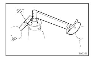
(c) Using SST to hold the flange, tighten the nut.
