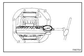
Using a dial indicator, measure the ring gear backlash. Backlash: 0.13 - 0.18 mm (0.0051 - 0.0070 in.)
