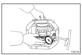
(c) Using a dial indicator, measure the side gear backlash while holding one pinion gear toward the differential case.
