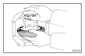
(e) Select a ring gear teeth side plate washer so that is no clearance between the outer race and case.
