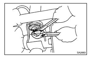
(b) Hold the shock absorber and remove the lower mounting nut, shock absorber, 3 cushions and 4 retainers.
