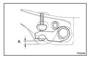
(b) Measure the dimension "A" between the anchor arm bolt end and the frame as shown.
