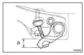
(c) Loosen the anchor arm bolt until the spring tension is free and measure the anchor arm bolt "B".
