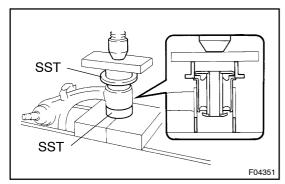
(c) Using SST, a steel plate and press, install a new bushing. SST 09316–20011, 09710–28012 (09710–07062)
