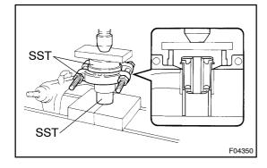
(b) Using SST, a steel plate and press, remove the bushing. SST 09527–17011, 09710–28021 (09710–08031), 09950–00020
