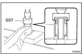
(c) Using SST and a press, install a new bushing. SST 09726–36010
