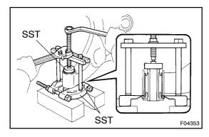
(b) Using SST, remove the No. 1 bushing. SST 09710–30021 (09710–03101), 09950–00020, 09950–00030, 09950–40011 (09957–04010)
