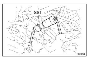
(b) Using SST, install a new bushing. SST 09631-32020, 09830-36010
