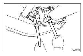
(b) Remove the 2 bolts and nuts from the leading arm on the axle housing side.
