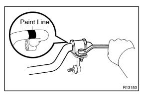
Remove the 4 bolts, 2 covers, 2 cushions and 2 stabilizer (c) bar links from the stabilizer bar.
