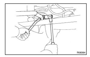
Remove the bolt, nut and stabilizer bar from the axle
