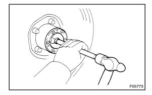
(b) Using a brass bar and hammer, strike the center part of the axle shaft to remove the 6 cone washers.
