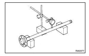
(b) Using a dial indicator, check the runout of axle shaft.
