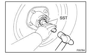
(b) Using SST and a hammer, install a new oil seal into the hub.
