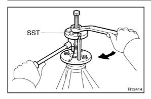
(c) Using SST, install the companion flange. SST 09950 -30010 (09951 -03010, 09953 -03010, 09954-03010, 09955 -03030, 09956 -03040)
