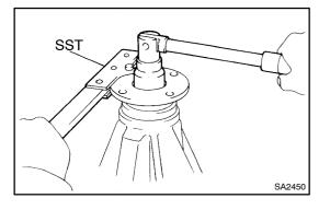
(d) Using SST to hold the flange and adjust the drive pinion preload by tightening the nut. SST 09330 -00021
