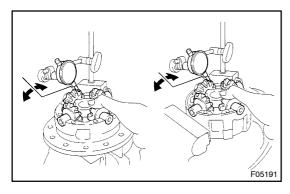
(e) Using a dial indicator, measure the side gear backlash holding the side gear and spider.
