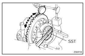
(i) Using a dial indicator, adjust the ring gear backlash until it is within the specification.
