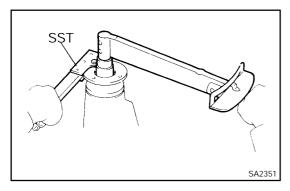
(c) Using SST to hold the flange, tighten the nut. SST 09330-00021
