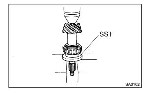
(b) Using SST and a press, install the rear bearing onto the drive pinion.
