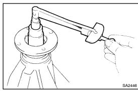
(e) Using a torque wrench, measure the preload.
