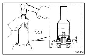
(b) Using SST and a hammer, install a new oil seal. SST 09214-76011
