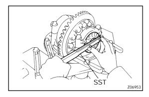
(b) Then loosen them to the point where the adjusting nuts can be turned by SST.
