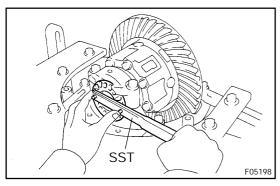
(e) While turning the ring gear, use the SST to fully tighten the adjusting nut on the drive pinion side. After the bearings are settled, loosen the adjusting nut on the drive pinion side.
