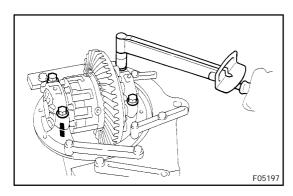
(j) Torque the 4 bearing cap bolts.
