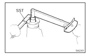
If the preload is less than the specification, retighten the nut with a force of 13 N·m (130 kgf·cm, 9 ft·lbf) at a time until the specified preload is reached.
