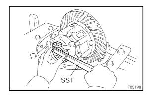
(h) Using SST, torque the adjusting nut 1 – 1.5 notches from the zero preload position.
