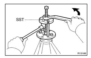
(c) Using SST, remove the companion flange. SST 09950 -30010 (09951 -03010, 09953 -03010, 09954-03010, 09955 -03030, 09956 -03040)
