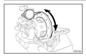
(f) Using a dial indicator, measure the differential case run-
