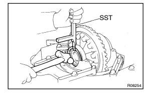
(c) Using SST and a hammer, remove the plate washers. SST 09504 –22011
