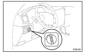
(c) Turn the differential lock control switch to the RR position and lock the rear differential.
