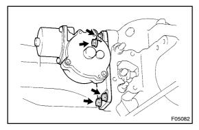
(g) Tighten the 4 bolts uniformly, a little at time.
