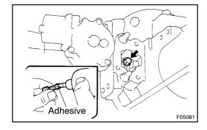
(e) Coat the threads of the set bolt with adhesive.
