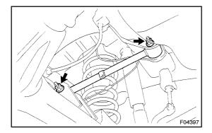
(c) Remove the 2 nuts, washers, bolts, and upper control arm.
