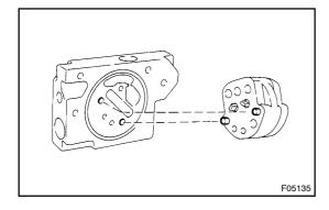
(b) Align the pin of pump sub -assembly and housing.
