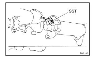
(b) Using SST, disconnect the outlet fluid line from the height control accumulator.
