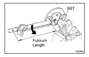
(c) Using SST, install the gas chamber.
