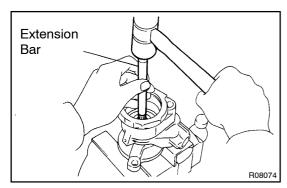
(b) Using an extension bar and hammer, tap out the shaft with the bearing.
