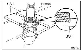
(c) Using SST, press out the gear. SST 09527 –10011
