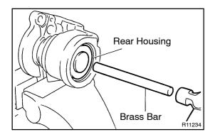
(b) Using a brass bar and hammer, tap the housing so that the spring force of the wave washer pushes the housing forward.
