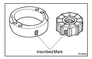
If it is more than the maximum, replace the plate and/or rotor with the one having the mark corresponding to the mark stamped on the cam ring.
