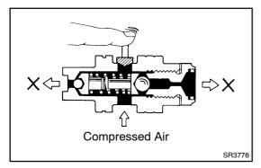
(b) Check the flow control valve for leakage. Close one of the holes and apply compressed air 392 - 490 kPa (4 - 5 kgf/cm, 57 - 71 psi) into the opposite side hole, and confirm that air does not come out from the end holes.
