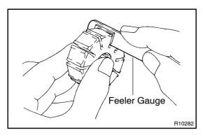
(b) Using a feeler gauge, measure the clearance between the rotor groove and plate.
