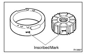
If it is more than the maximum, replace the plate and/or rotor with the one having the same mark stamped on the cam ring.
