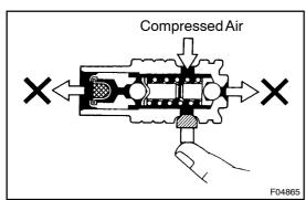
(b) Check the flow control valve for leakage. Close one of the holes and apply compressed air 392 - 490 kPa (4 - 5 kgf/cm<sup>2</sup>, 57 - 71 psi) into the opposite side hole, and confirm that air does not come out from the end holes.
