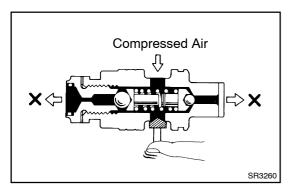
(b) Check the valve for leakage. Close one of the holes and apply compressed air 392 - 490 kPa (4 - 5 kgf/cm , 5 7 - 71 psi) into the opposite side hole, and confirm that air does not come out from the end holes.
