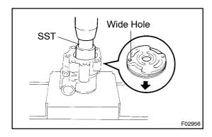
(c) Using SST, press in the plate. SST 09238 -47012
