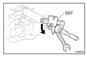
(b) Using a spanner, hold the steering rack steadily and using SST, remove the rack end.
