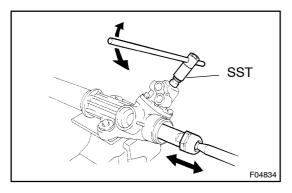
(d) Using SST, turn the control valve shaft right and left 1 or 2 times.
