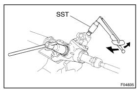
(f) Using SST and a torque wrench, tighten the cap until the preload is within specification.
