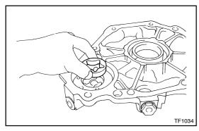
4. REMOVE DRIVEN ROTOR FROM REAR EXTENSION HOUSING
