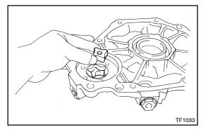
3. REMOVE DRIVE ROTOR FROM DRIVEN ROTOR
