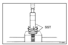
(b) Using SST and a press, install a new rear output shaft dust deflector.
