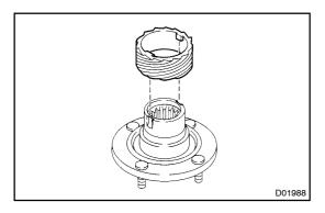
(d) Remove the speed sensor drive gear from the companion flange.
