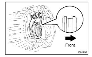
(b) Remove the front drive clutch sleeve, No.2 shift fork, 2 plate washers and compression spring.
