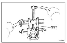
(e) Using SST, remove the dust deflector from the companion flange.
