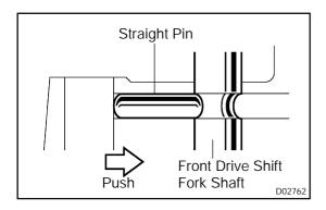
After installing the front drive shift fork shaft, push the straight pin in the groove of the front drive shift fork shaft, as shown in the illustration.
