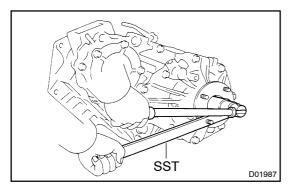
(b) Using SST to hold the flange, remove the nut and O -ring. SST 09330 -00021
