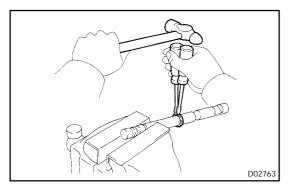
(b) Using 2 screwdrivers and a hammer, drive out the snap ring from the front drive shift fork shaft.
