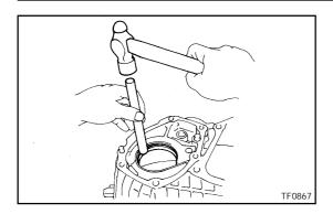
(b) Using a brass bar and hammer, remove the bearing outer race (for the output shaft).
