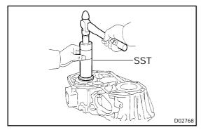
(c) Using SST and a hammer, drive in a new oil seal. SST 09316-60011 (09316-00011, 09316-00031)
