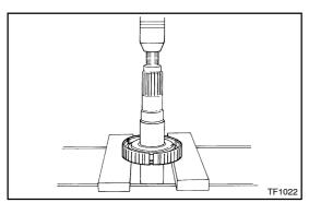
(b) Using a press, remove the clutch hub.
