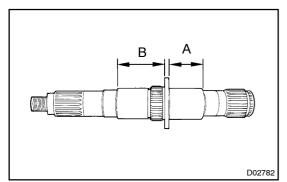
(b) Using vernier calipers, measure the length of the output shaft journal.
