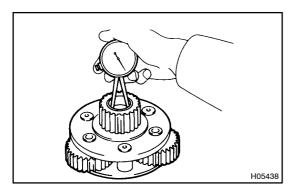
(b) Using a caliper gauge, measure the bushing bore of the planetary gear No.3.
