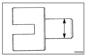
(b) Inspect the outer clutch for wear or damage. If necessary, replace the drive shaft.
