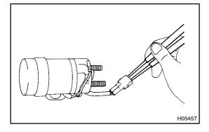
(b) Using an ohmmeter, measure the resistance between connector terminals.
