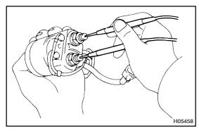
(c) Using an ohmmeter, check for no continuity between the terminals with the plunger released.
