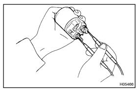
(c) Using an ohmmeter, check for no continuity between the magnet switch terminal and motor lead wire terminal with plunger released.
