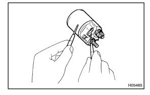
(b) Using an ohmmeter, check for continuity between the base lead wire terminal and magnet switch body.If there is no continuity, replace the magnet switch.
