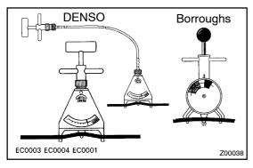
(c) Using a belt tension gauge, measure the belt tension.
