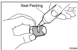
(c) Apply seal packing to 2 or 3 threads of the engine drain plug.
