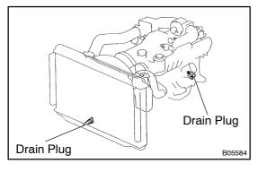
(b) Loosen the radiator drain plug (on the left side of the radiator lower tank) and engine drain plug (on the left side of the cylinder block), and drain the coolant.
