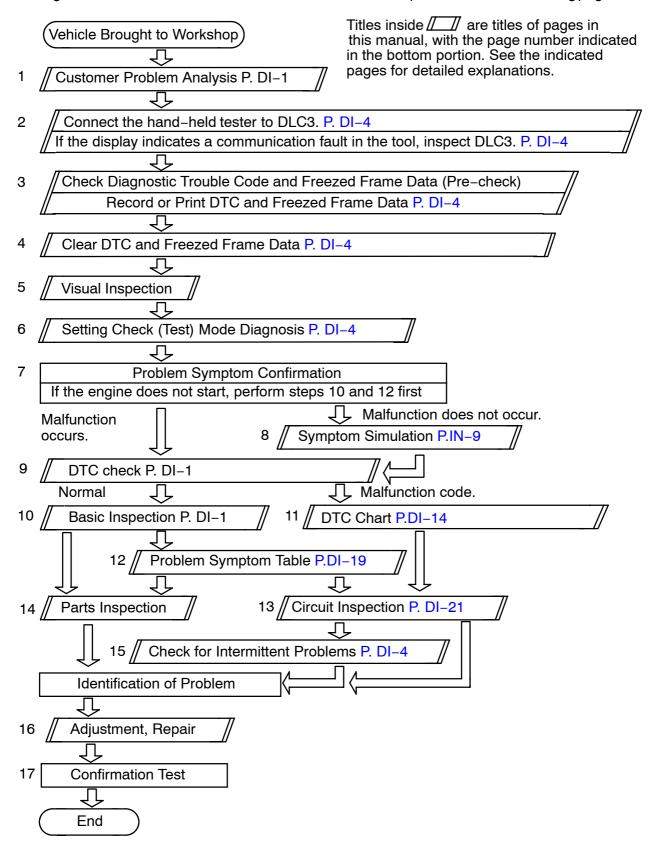
When not using hand -held tester, troubleshoot in accordance with the procedure on the following pages.
