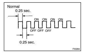
(3) Read the diagnostic trouble code from check engine warning light.
