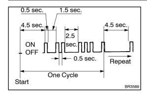
As an example, the blinking patterns for codes; normal, 12 and 31 are as shown on the illustration.
