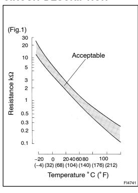
The water temperature sensor senses the coolant temperature. A thermistor built into the sensor changes the resistance value according to the coolant temperature. The lower the coolant temperature, the greater the thermistor resistance value, and the higher the coolant temperature, the lower the thermistor resistance value (See Fig.1).
