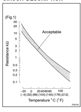
The fuel temperature sensor senses the fuel temperature. A thermistor built into the sensor changes the resistance value according to the fuel temperature. The lower the fuel temperature, the greater the thermistor resistance value, and the higher the fuel temperature, the lower the thermistor resistance value (See Fig.1).
