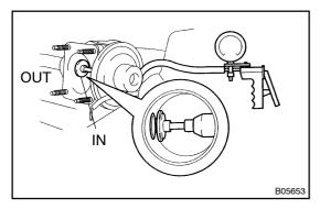
(b) Under the condition of applying the vacuum to the diaphragm chamber, check if there is ventilation between IN and OUT.
