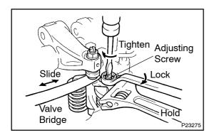
(f) Tighten the adjusting screw on the valve bridge, and lock the adjusting screw with the lock nut when the resistance of the feeler gauge begins to get stronger.
