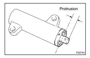
(c) Measure the protrusion of the push rod from the housing end.
