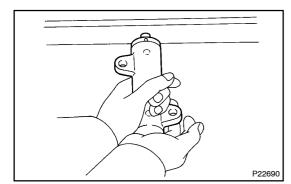
(b) Hold the tensioner with both hands and push the push rod strongly as shown to check that it doesn't move.If the push rod moves, replace the tensioner.
