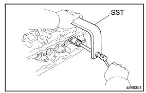
(c) Using SST, compress the valve spring and place the 2 keepers around the valve stem.
