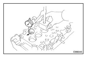
(c) Using a dial indicator, measure the protrusion of the combustion chamber from the cylinder head.
